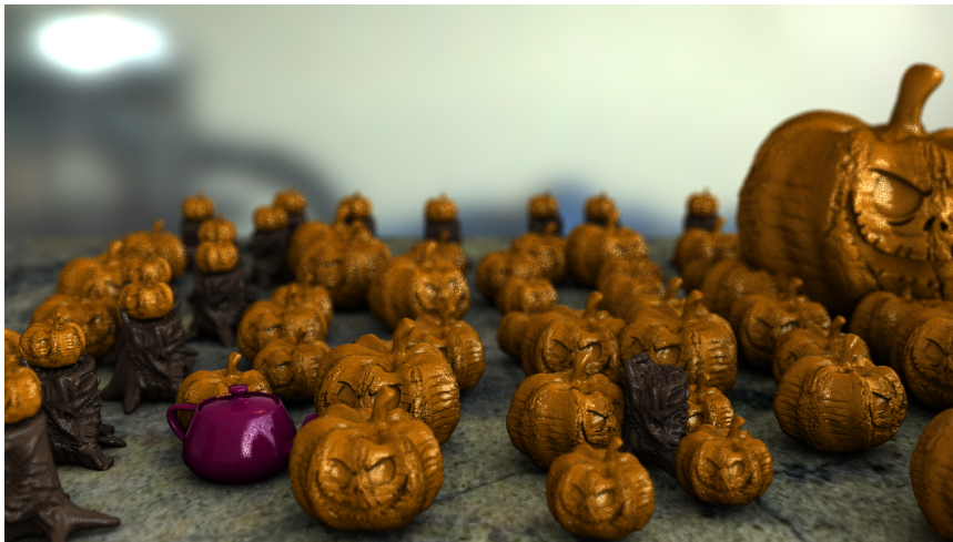
Figure 1.1: The "Party" scene with vector displacement mapped surfaces rendered using the proposed method. The rendering time is 77ms/frame on an AMD FirePro W9100 GPU. Instancing is not used to stress the rendering algorithm. If pre-tessellated, the geometry requires 52GB memory.
